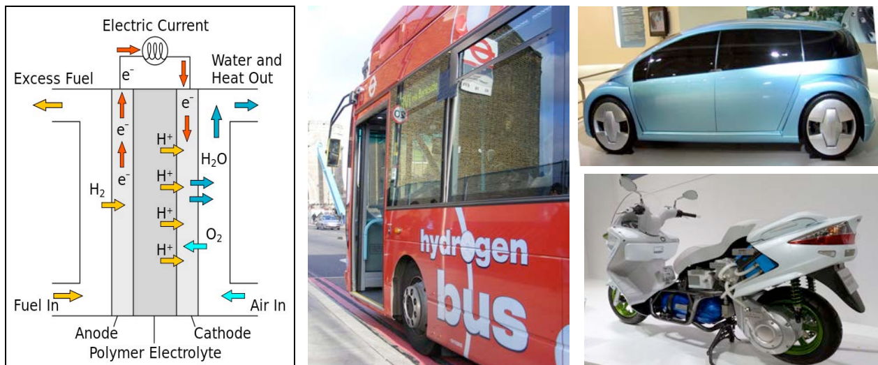
Figure 5.14: The electrochemical processes showing how hydrogen fuel is combined with oxygen generating heat energy along with water as a waste product. Some vehicles that use the fuel cell include buses (photo is a hydrogen fuel bus on Tower Bridge London, photo by Sludge G.), cars (The Toyota Fine N car based on fuel cell technology, photo by Chris 73, CC BY-SA 3.0) and motorcycles (Suzuki Burgman Fuel Cell cutaway model shown here, Photo by Mario CC BY-SA 3.0).
