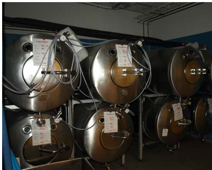
Figure 7.16 Fermentation of grape juice produces CO 2 as a byproduct. Fermentation tanks have valves so that the pressure inside the tanks created by the carbon dioxide produced can be released.
