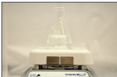
(D) The solution is cooled to room temperature, leading to the formation of large crystals.
