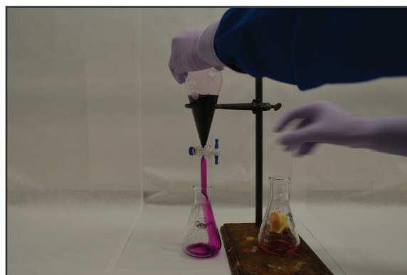
(D) The top phase is then drained into a clean container.
