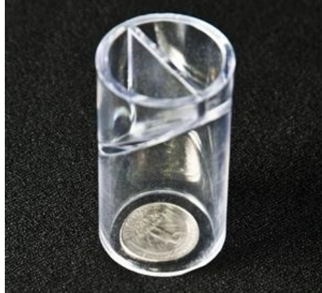
Figure 3.18 – This is a small parts tester (or choke tube). If an item/toy fits inside, it's a choking hazard. 59
