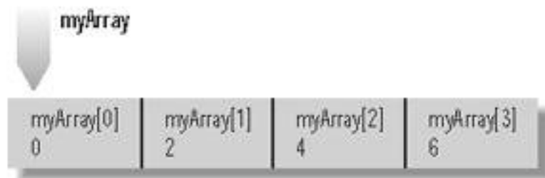
Figure 2.16: Values assigned to elements by index
