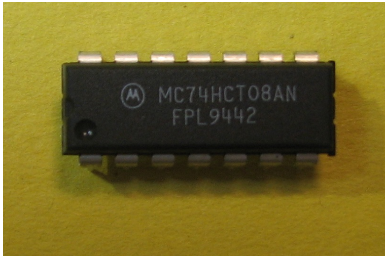
Figure 4-6: 7408 chip, circle indicates top of chip.
