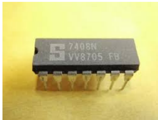
Figure 4-7: 7408 chip, notch indicates top of chip.
