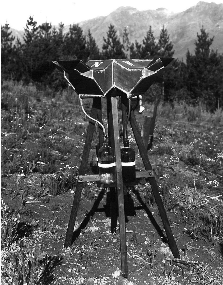
Figure 16. A vectopluiometer. This raingauge was designed by Henry Fourcade to measure the inclination (the departure from vertical) of rain and its bearing (the direction from which it arrives), for the full characterisation of rainstorms.
