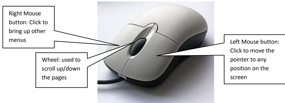
Figure 3.7: Typical mouse and the functions of its buttons and wheel
