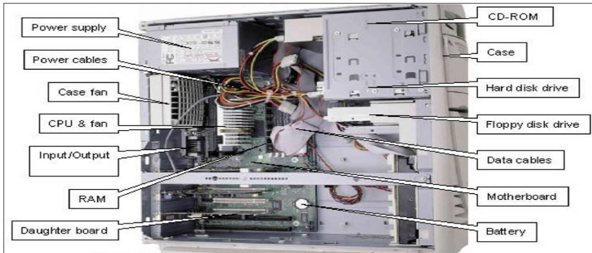
Figure 3.38: Components inside the System Unit
