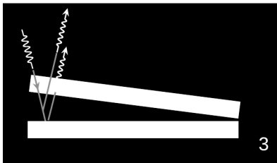
ab / 1. Interference in an air wedge. 2. Side view. 3. If the wedge is thicker than the coherence length of the light, the interference pattern disappears.
