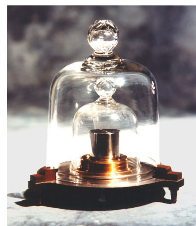
f / A duplicate of the Paris kilogram, maintained at the Danish National Metrology Institute. As of 2019, the kilogram is no longer defined in terms of a physical standard.
