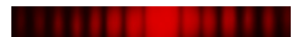
w / Single-slit diffraction of red light. Note the double width of the central maximum.
