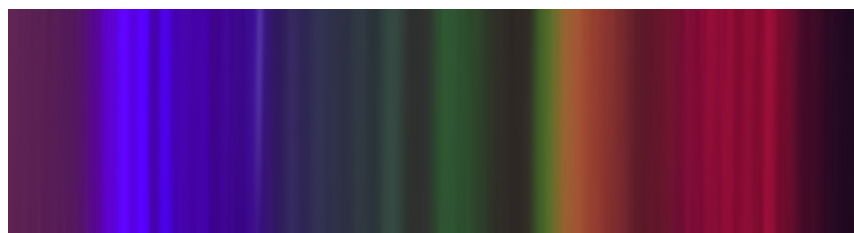
a / Visible spectrum of N_2 . Violet is on the left, red on the right.
