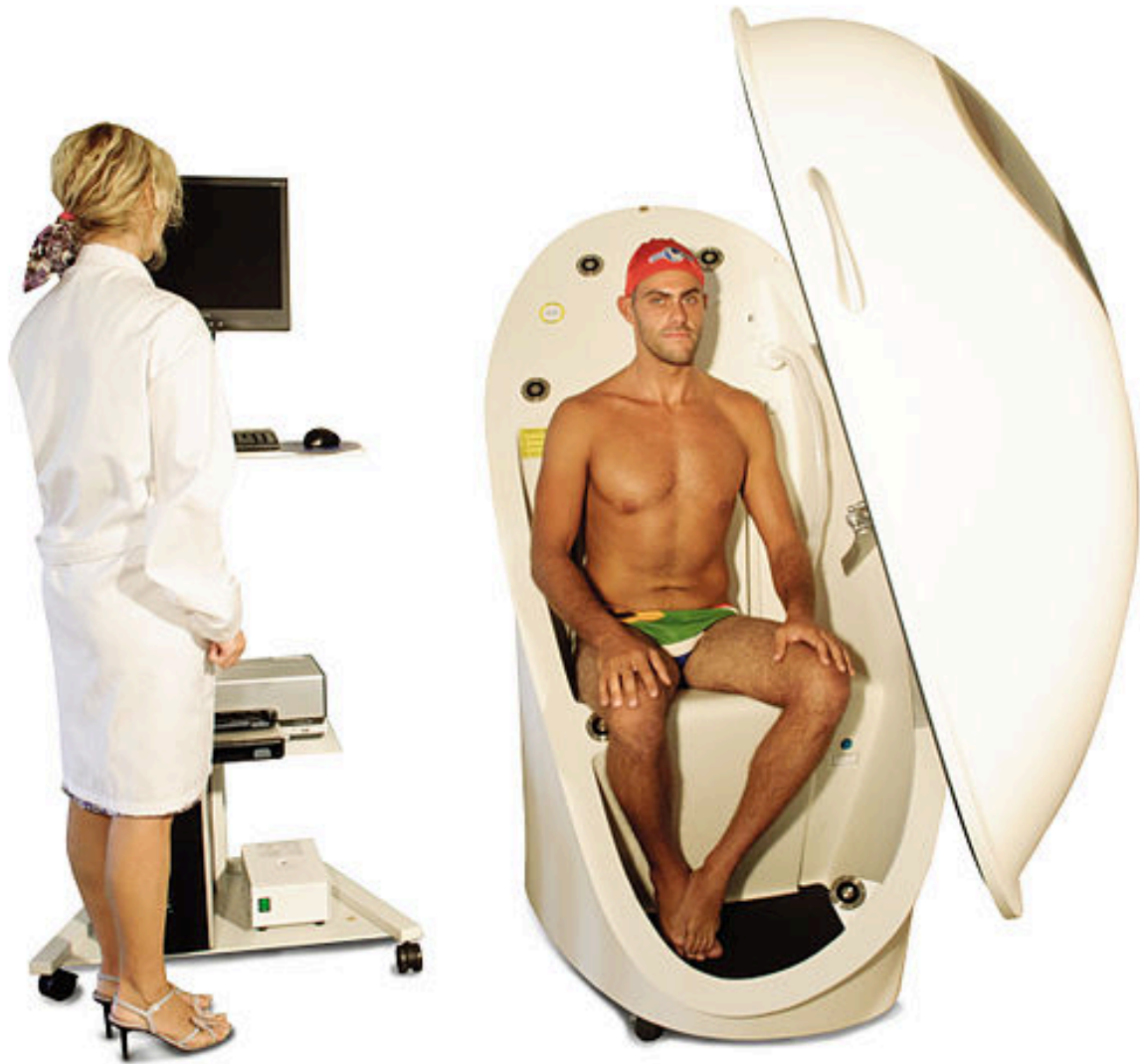
Figure 7.11. Body composition measurement with whole-body air displacement plethysmography (ADP) technology or BodPod
