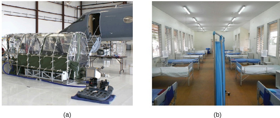
Figure 12.13 (a) The Aeromedical Biological Containment System (ABCS) is a module designed by the CDC and Department of Defense specifically for transporting highly contagious patients by air. (b) An isolation ward for Ebola patients in Lagos, Nigeria. (credit a: modification of work by Centers for Disease Control and Prevention; credit b: modification of work by CDC Global)
