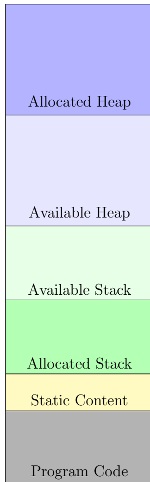
Figure 7.4.: Depiction of Application Memory. The details of how application memory is allocated and how the stack/heap “grow” may vary depending on the architecture. The figure shows stack memory growing “upward” while heap allocation grows “downward.” Allocation and deallocation may fragment the heap space though.
