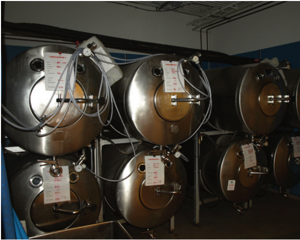
Figure 7 Fermentation of grape juice to make wine produces \text{CO}_2 as a byproduct. Fermentation tanks have valves so that pressure inside the tanks can be released.
