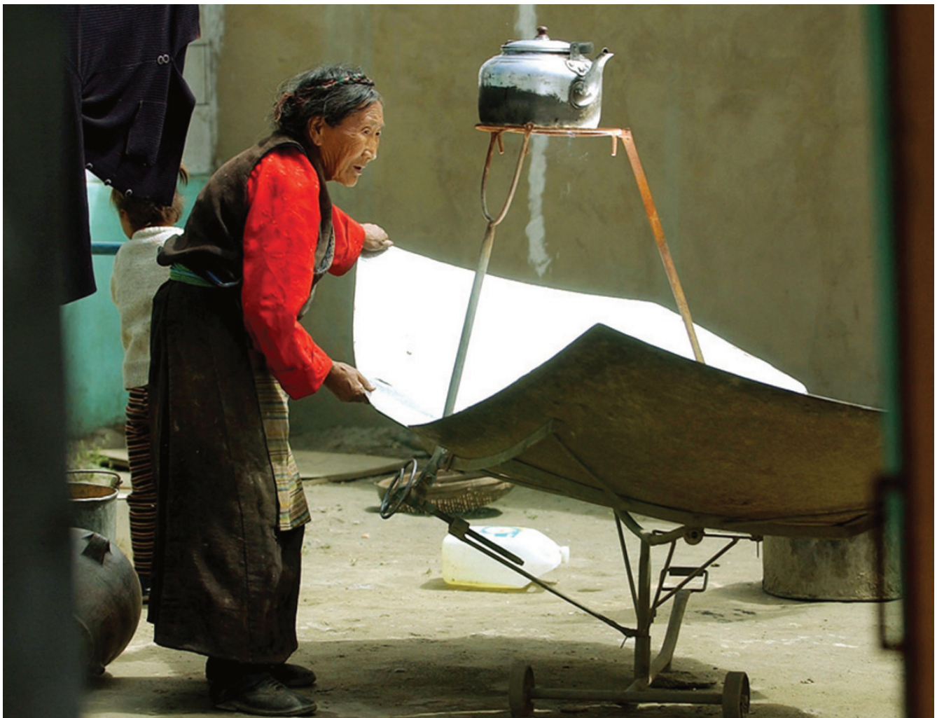
Figure 11.3: A woman in Tsetan, Tibetan Autonomous Region, China, uses a home-made solar cooker to boil water.
