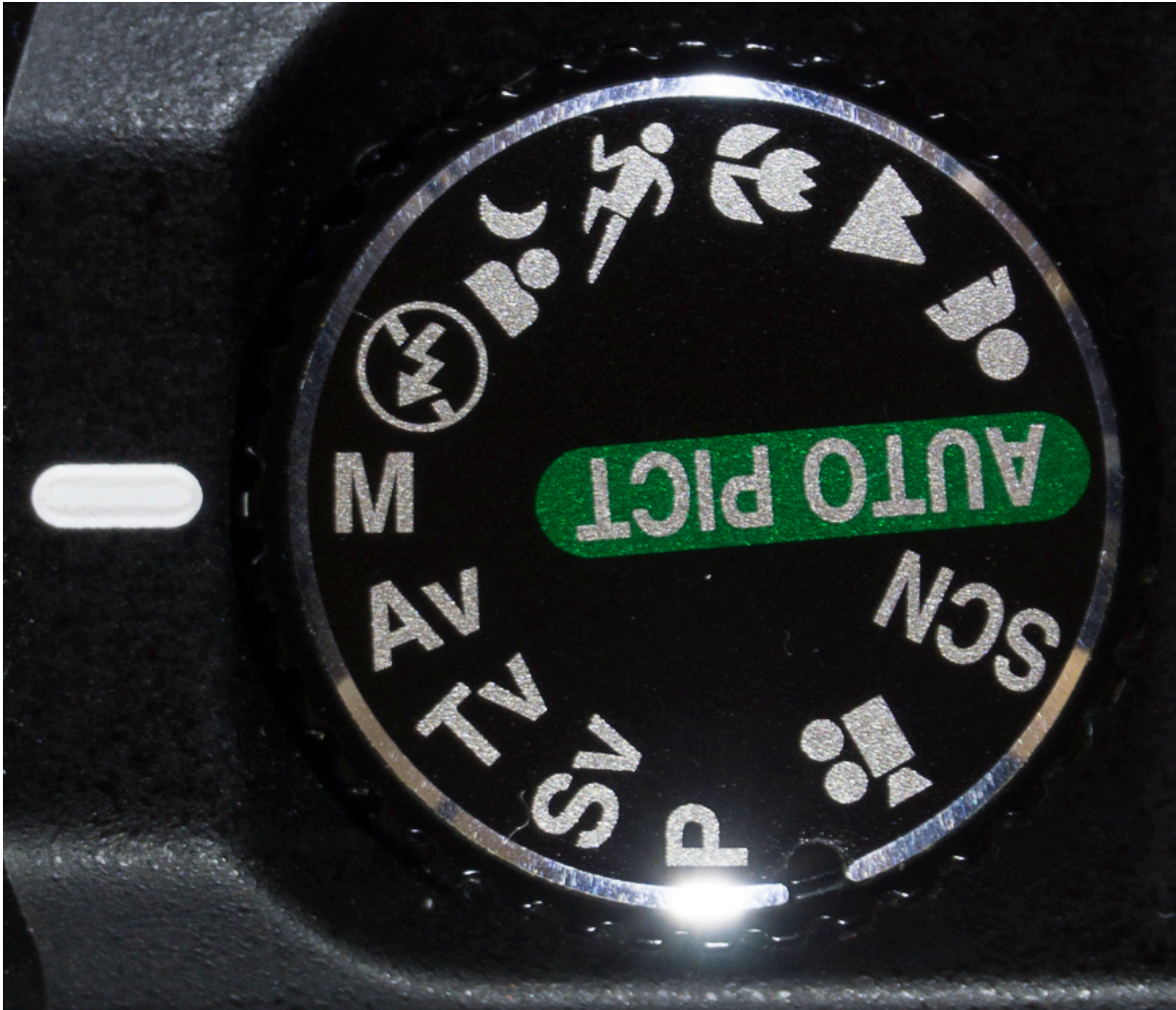
Figure 14-2. Mode dial on a DSLR camera includes manual, aperture priority (“Av”), shutter priority (“Tv”), ISO priority (“Sv”), and program (“P”) modes, along with various scene settings. For web work manual gives the greatest control and consistency.
