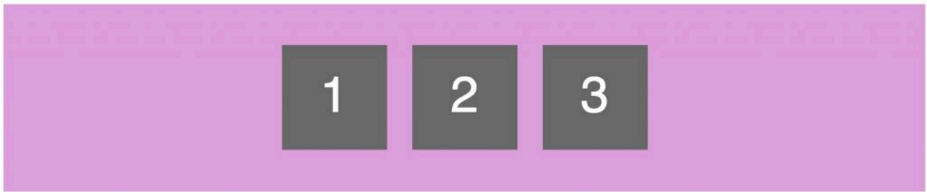
Figure 5-5. The “display: flex” style was applied to the plum-coloured div, and the enclosed paragraphs 1, 2, and 3 were aligned by setting the div to “justify-content: center” (horizontal) and “align-items: center” (vertical).
