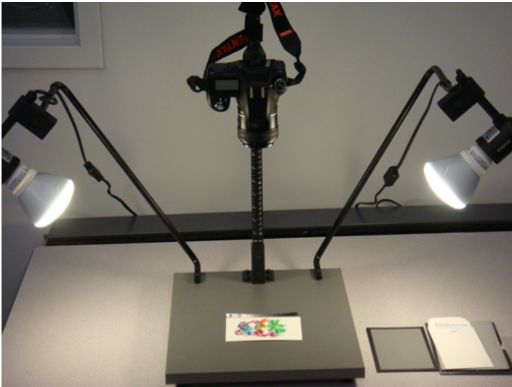
Figure 14-3. A 15% grey card (to right of table) is used to set manual exposure to 0 EV on this DSLR copy stand setup.
